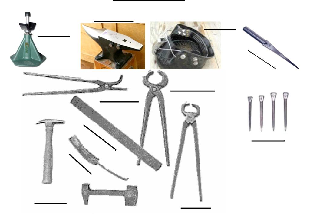
Buffer - The buffer is used to remove the end of the clenched nail, (turned over end of nail).
